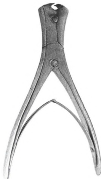
AO-INS-882 Wire Cutter 220 mm TC soft wire 2.5 mm hard wire 2.2 mm A550 01 091 0882 8698823350895
