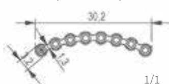
A110 03 351 1308 1,3 mm Maxillofacial Micro Orbital Curved Plate, 8 Holes, Thickness 0,5 mm
