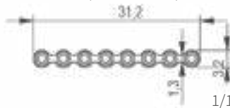
A110 03 212 0080 1,3 mm Maxillofacial Micro Straight Plate, 8 Holes, Thickness 0,5 mm
