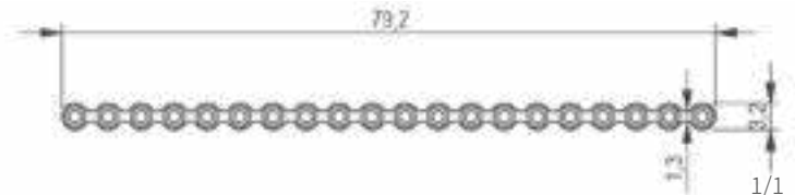
A110 03 212 0200 1,3 mm Maxillofacial Micro Straight Plate, 20 Holes, Thickness 0,5 mm
