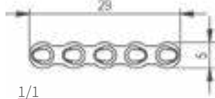
A110 03 321 2080 2,0 mm Mandibular Trauma Mini Locking Straight Compression Plate, 5 Holes, Thickness 1,0 mm
