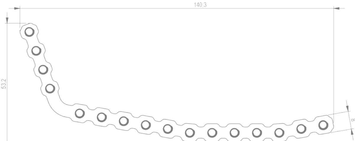
2,4 mm Mandibular Locking Reconstruction Double Angled Curved Right Plate
